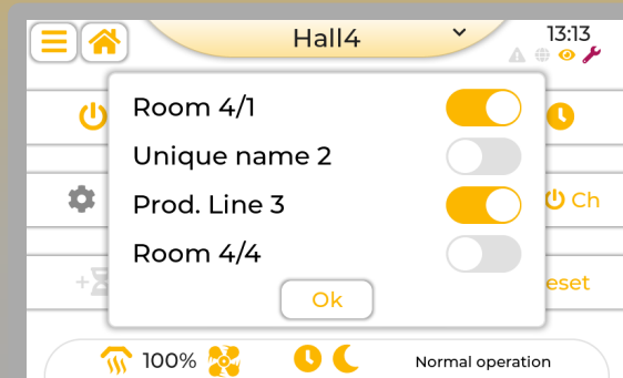
Max. 4 heater groups (channels) in each zone
